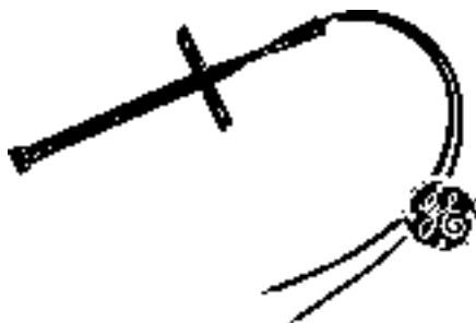
WB21X158 2 7/8" Long Probe G.E./Hotpoint Self Cleaning Oven Sensor. Resistance 16Ω, Increases with Temp. Complete with Ceramic Nuts. (Illustrated) WB21X5301 6" Long Probe G.E./Hotpoint Self Cleaning Oven Sensor. 1000Ω Plug in Block Connection.
