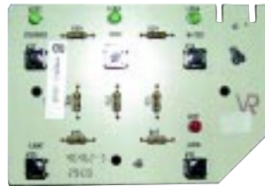
61003421 Admiral Switch Board. For water and ice in door.
